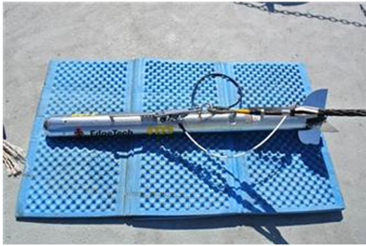
Fig. 4. 4125 Shallow water side scan sonar system towfish(EdgeTech).
